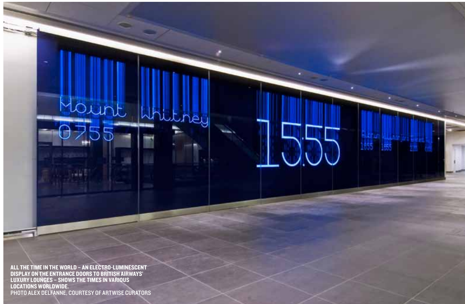
THE DISPLAY RELIES ON A CUSTOM-DESIGNED SEGMENTED TYPEFACE THAT IS LESS THAN HALF A MILLIMETRE THIN AND CAN BE CURVED.
